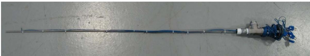
**Figure 5: Typical Thermocouple Tree for Storage Tank Temperature Measurement**
