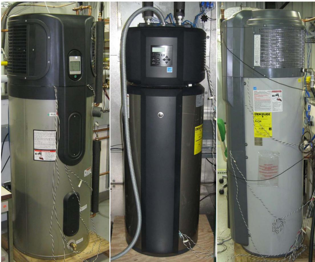
**Figure 3: HPWHs Tested in this Study**
